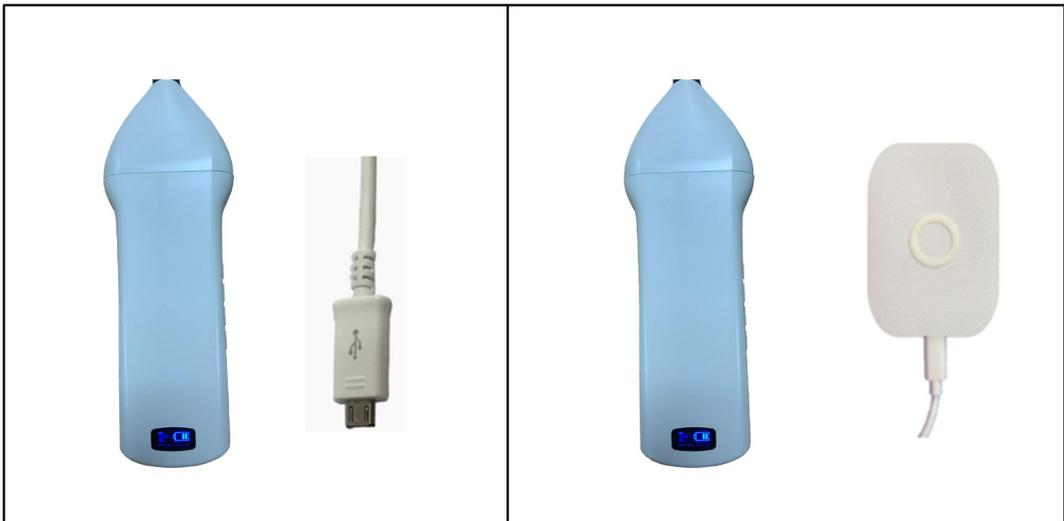
Figure 4-1 Charge the Probe
