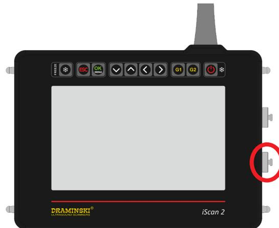
*Data transmission slot protecting plug*
